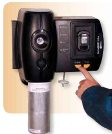
Bump testing ToxiRAE 3 with AutoRAE Lite Bump Test and Calibration Station
